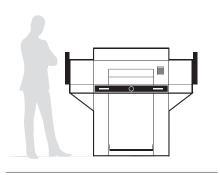
Dimensiones  $1370 \times 1070 \times 1400 \text{ mm}$  (Al x An x Pr)
